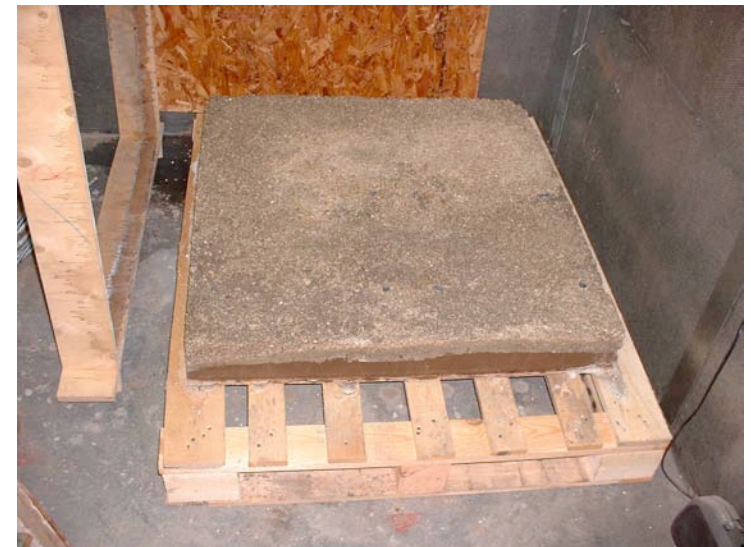
Photo 5: First cement side; composite slab removed from former
