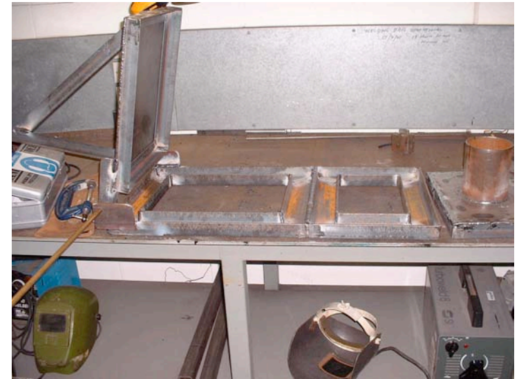
Photo 8: Steel top complete
