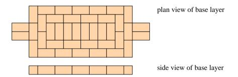
Subsequent layers of bricks are then laid on top of the base layer as shown in the following diagrams. Care should be taken to keep all walls vertical and straight.
