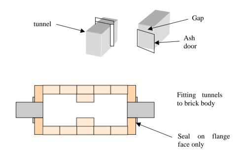
Diagram 13: steel tunnels and ash door
