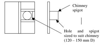
Diagram 12: chimney support plate and spigot
