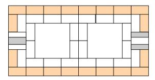
Diagram 14: incinerator outer case
